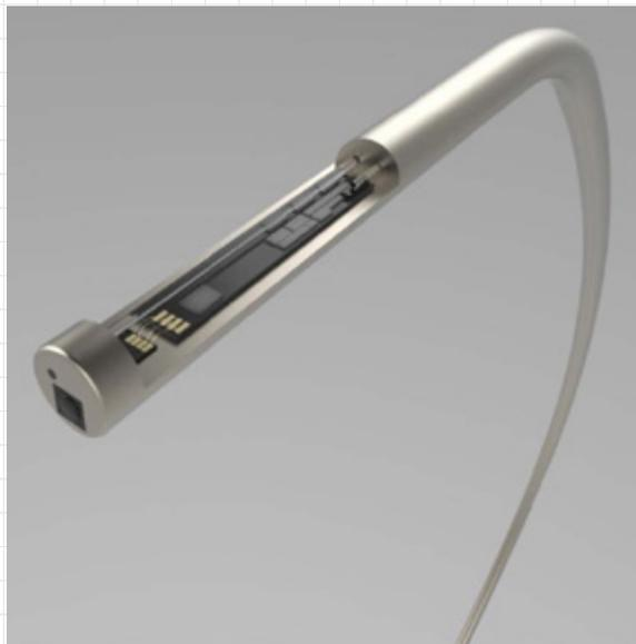
A 1mm diameter smart Guidewire with image sensor for surgical assistance in stent operations.
